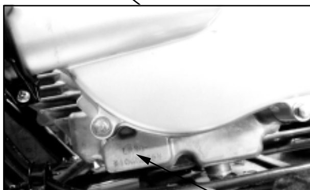
Location of Engine Serial Number
